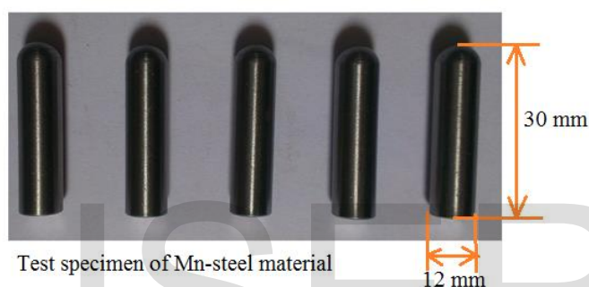
Figure 1. Image of test specimen samples made from Mn-steel material.
